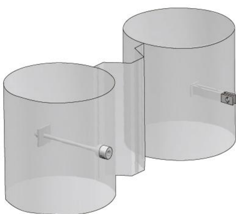
Pipe Pile Connections
